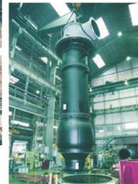
Brine recirculation pump for Ras Laffan MSF desalination plant, Qatar (Size: 1200mm, Driver: 3800kW)
