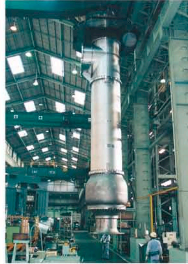
Cooling water pump for P.A.I. Shuaiba, Kuwait (Size:1400mm, Driver:1500kW)
