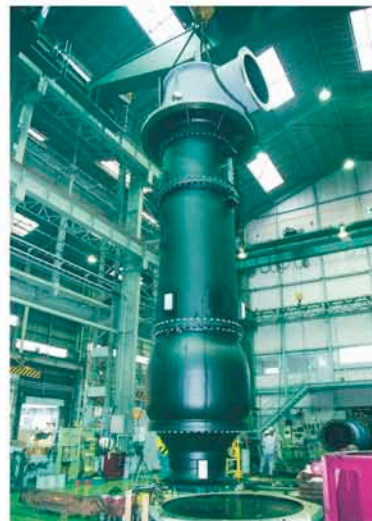
Brine recirculation pump for Ras Laffan MSF desalination plant, Qatar (Size:1200mm, Driver:3800kW)
